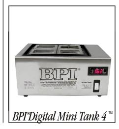
The system has an 1/0 circuit breaker switch .and a temperature control, with indicator lamp. The lamp in the temperature controller indicates when the unit into a properly grounded 120 volt electrical receptacle (The 220 volt model is shipped without a plug and requires a qualified technician for installation). Plug temperature probe into back of
