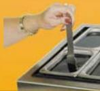
1. 93-96°C (200-205°F) is the optimum tinting temperature. It allows the correct migration of the different size pigments that make up a typical BPI® tint. The lens material will not accept the tints correctly unless this temperature is maintained.
